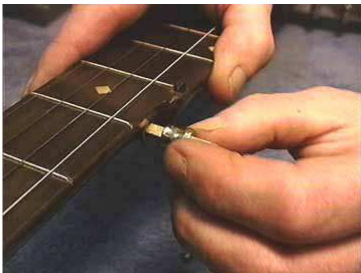
And place a single drop of oil on the shaft as it enters the housing:
