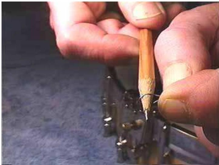
Some tailpieces have hooks that are hard to reach, or that don't hold the loops too well until the string is tuned. Bend the loop to fit the contour of the tailpiece if necessary. Hold the end down to the pointy end of a pencil and just roll the loop around:
