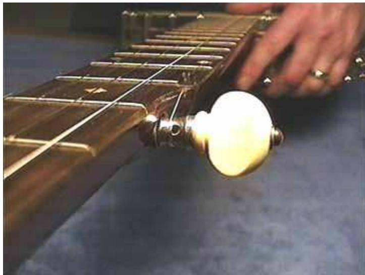
This innocent looking fellow can cause a lot of headaches. If the peg is loose in the neck, a light tap with a plastic hammer should seat it in its tapered hole. If that doesn't work, a trip to your local banjo mechanic may be in order.
