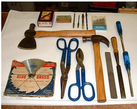
John Primble pocket knife box, green saw nut box held a dozen two piece saw nuts marked 15 cents, brace bits, Set of Bluegrass drill bits, Bluegrass hatchet, Bluegrass circular saw blade, Bluegrass tin snips, 16oz. Pine Knot hammer, Bluegrass shoe rasp, Pine Knot 3/4 chisel, and a pair of Bluegrass blue plastic handled 3/8" chisels with Logos in white.
