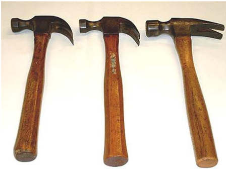
From left: 20oz Bluegrass Hammer from about 1940, 20oz Bluegrass Hammer from about 1930, 28oz Bluegrass Hammer from about 1970.
