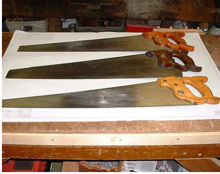
From the top: Belknap Master Mechanic Saw No. 549, Belknap Handsaw with W. B. Belknap & Co. on medallion (1860-1880), Belknap Cyclone Handsaw.
