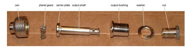
OK, you get the idea. By the way, the annular ring gear in the can has 20 teeth. If the annulus is held stationary and the sun gear is used as the input, the planet carrier will be the output. The gear ratio in this case will be 1/(1+A/S), or 1/(1+20/6), or 1/4.33.
