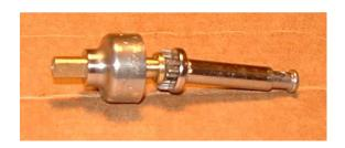
OK, here you see the planet gears in place on the carrier/output shaft. The sun gear is inside the triangle formed by the 3 planet gears.
