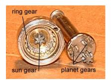
This view shows the input shaft and sun gear in the "can" (I don't know what else to call it). Note also the annular gear with its 20 teeth on the inside of the can. The sun gear, with 6 teeth, is in the center. On the right is the output shaft with the 3 6-tooth planetary gears.
