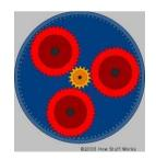
In this gear system, the yellow gear (the sun) engages all three red gears (the planets) simultaneously. All three are attached to a plate (the planet carrier), and they engage the inside of the blue gear (the ring, sometimes called the annulus) instead of the outside. Because there are three red gears instead of one, this gear train is extremely rugged. The output shaft is attached to the blue ring gear, and the planet carrier is held stationary -- this gives the same 6:1 gear ratio.
