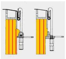
Depending on the model, there were either of three or four plies: three plies of 1/4" maple to make up a 3/4" rim machined down for one-piece flange models, and four plies of 1/4" rim to make up the heavy rim used for tube-and-plate models. All of the laminate ends were taper-cut, a method of angling the joining ends of each laminate so that they would overlap rather than joint flat end-to-end.
