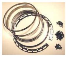
Gilbson's spring-loaded ball-bearing tone chamber system was a marvelous engineering feat of wood and metal parts. The assembly included (left to right) a grooved stretcher band, exterior tone chamber rim, tone tube with integral lip and arched upper ring, tube and plate assembly, 24 ball bearings, 24 coil springs, and 48 flat washers. Each spring was rated at 460 pounds per inch.
