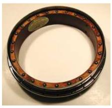
With all the springs in place, the rim is finally ready to have the tone tube installed. The assembly of these rims was very time consuming and it is no wonder that the Company eventually favored a one-piece tone chamber and lastly, a one-piece cast flange.
